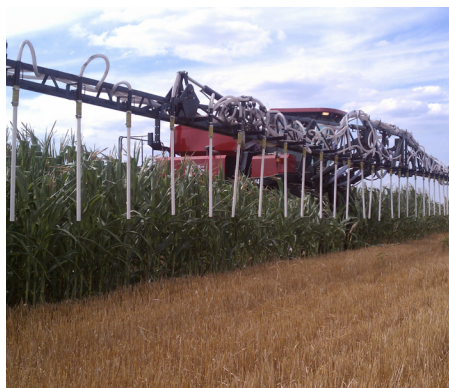
The VanTilburgs fashioned a cover crop seed planter from a highboy sprayer.
