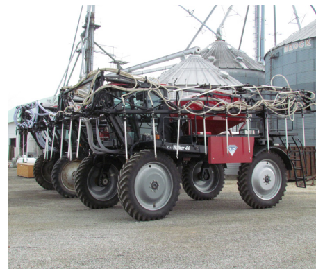
The VanTilburgs fashioned a cover crop seed planter from a highboy sprayer.
