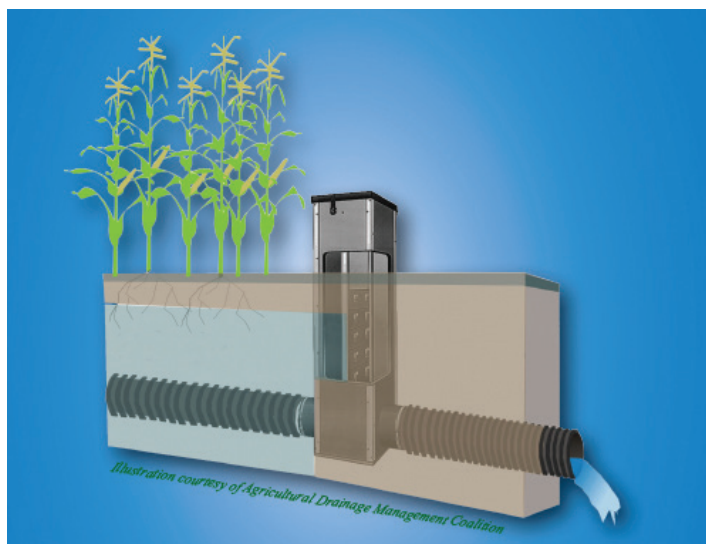
Stop logs are controlled within this control box to allow the rise and fall of the water table with the tile lines allowing plants to absorb more water. Image courtesy of USDA NRCS.
